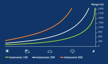
Autonomic comes in three models, each with a different laser output power. The Autonomic 100, 200 and 500. Choosing the right model is essential in order to generate a laser projection with sufficient contrast for effective bird dispersal.
